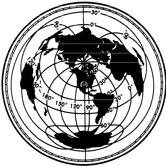
Figure 2-17. Azimuthal Equidistant Projection with Point of Tangency Lat 40°N, Long 100°W.
