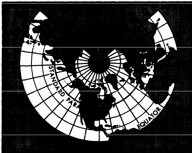
Figure 2-24. Simple Conic Projection of Northern Hemisphere.
